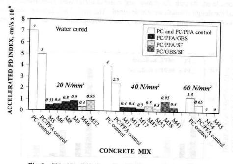
Fig.5. Chloride diffusion of multi-component binder concrete
