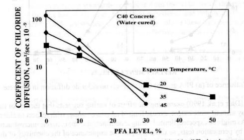
Fig.4. Influence of exposure temperature on chloride diffusion in concrete
