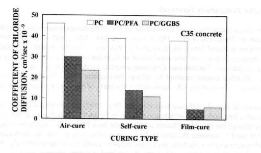
Fig.8. Chloride diffusion of self-cure concrete
