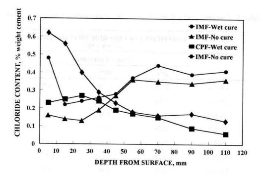
Fig.11. Chloride concentration profiles in CPF concrete under hot/dry exposure conditions (Price and Widdows, 1992)
