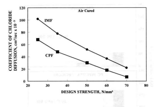
Fig.10. Influence of CPF on chloride diffusion in concrete
