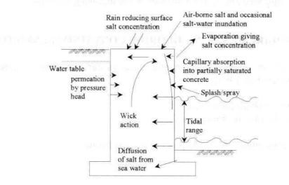
Fig 1. Mechanisms of chloride ingress into concrete (Concrete Society, 1996)
