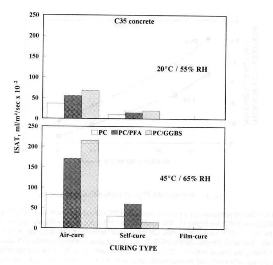
Fig.9. Effect of temperature on ISA of self-cure concrete
