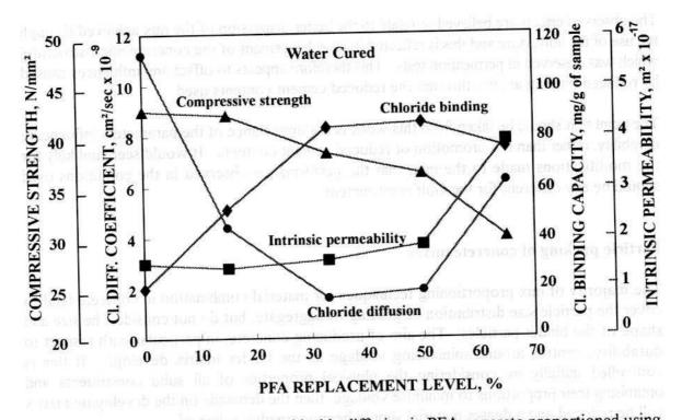
Fig.7. Influence of various factors on chloride diffusion in PFA concrete proportioned using particle packing method
