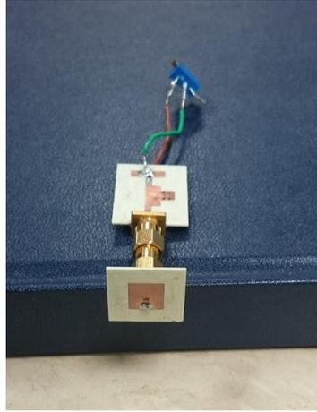
Figure 5.21 Fabricated 5.2 GHz rectenna
