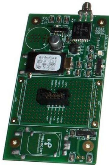
Figure 4.22 Powercast Evaluation Board (P2110-EVB) [95]
