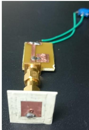
**Figure 5.20 Fabricated 2.43 GHz rectenna**
