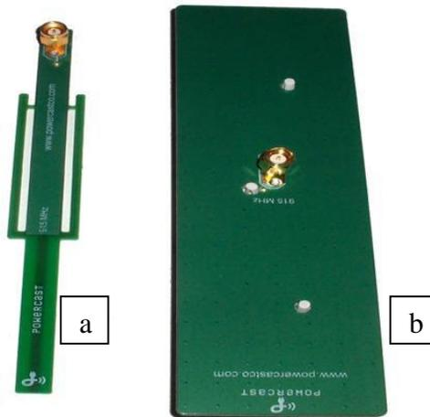
Figure 4.23 Powercast antennas (a) Dipole antenna (b) Patch antenna [93]
