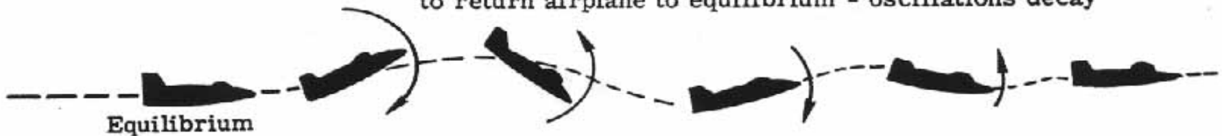
(a) Statically and dynamically stable.
