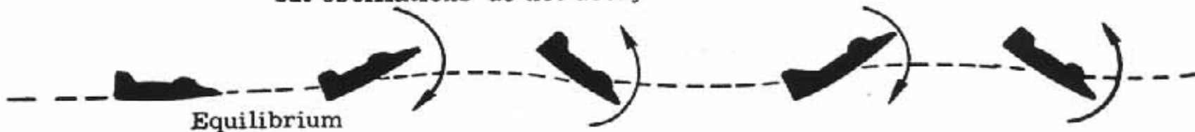
(b) Statically stable; neutral dynamic stability.
